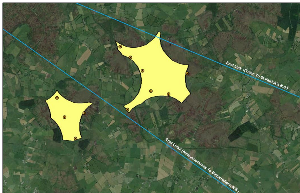
Figure 8. Telecommunication links that cross over/near the proposed wind farm site.
